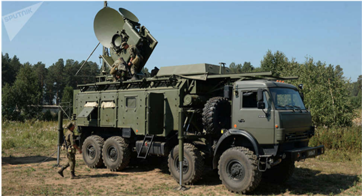
Figure 8 - Krasukha-4 A Russian mobile electronic warfare system used to jam radar. Image credit: Sputnik News. 190
