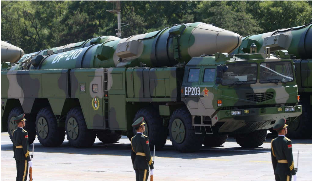
Figure 3 - DF-21 MRBM Missile version upon which the SC-19 is likely based, mounted atop a TEL. Image credit: Defence Blog. 48
